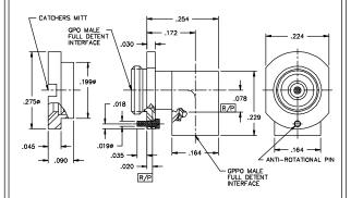
1. TIGHTEN FRONT NUT TO BULKHEAD HOUSING WITH 6lbs/in MAX.
